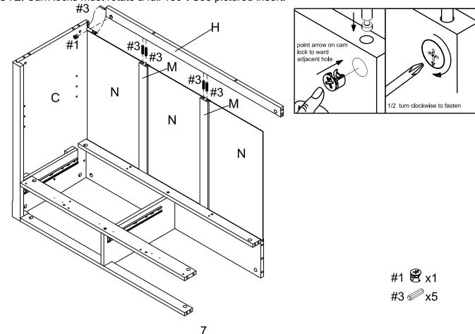
Step 7. Attach left panel (part B) to assembled unit (parts D, E, F, G, H & N) using wood dowels (part #3) and cam locks (part #1).
