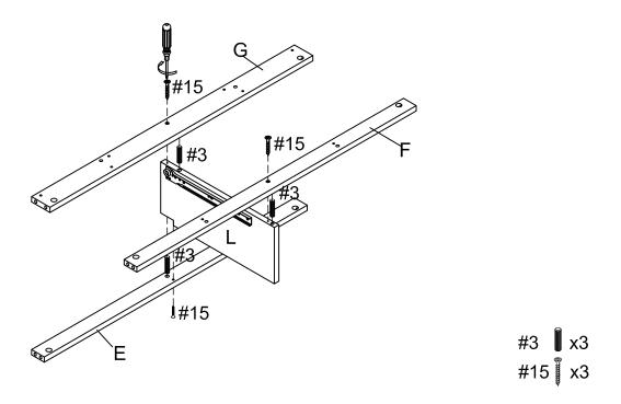
Step 4. Attach assembled unit (parts E, F, G & L) to right panel (part C) using wood dowels (part #3) and cam locks (part #1). Attach back top panel (part D) to right panel (part C) using wood dowel (part #3) and cam locks (part #1).
