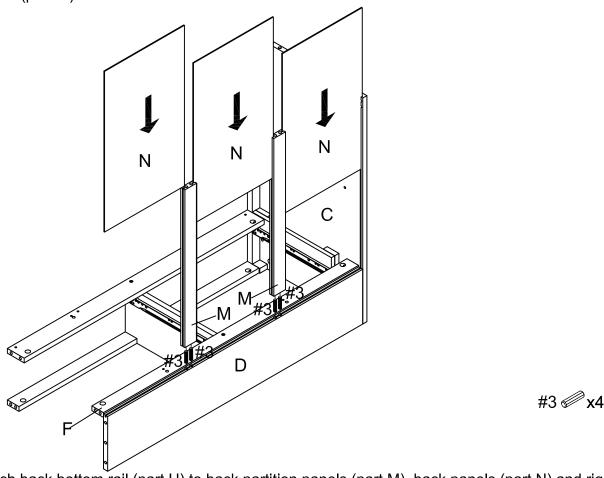
Step 6. Attach back bottom rail (part H) to back partition panels (part M), back panels (part N) and right panel (part C) using wood dowels (part #3) and cam lock (part #1).
