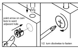
Step 15. Attach left door panels (part V) and right door panels (part W) by placing bottom pin hinge (pre-installed in door) in the pre-drilled hole of bottom panel (part I). Then depress the top spring-loaded pin hinge so it can be placed in the pre-drilled hole of front middle rail (part G). Place shelf holders (part #7) into desired position.
